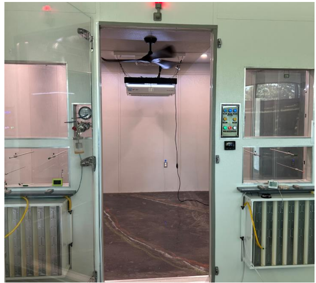
Figure 3: The 30 m 3 bioaerosol testing chamber at ARE Labs adheres to AHAM AC-5 standards and ASHRAE 241 criteria. The chamber is equipped with HEPA filtered air in/out, multiple bio aerosol sampling ports, decontamination, and pressure balance.
