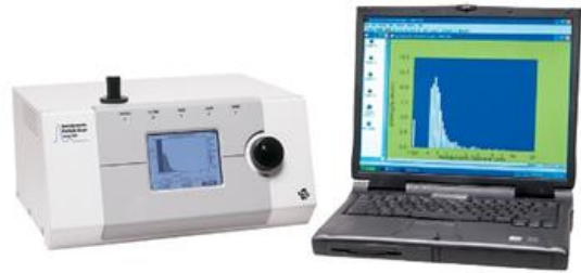
Figure 10. TSI Aerodynamic Particle Sizer (APS) model 3321 used to measure total particle concentration and particle size distribution of the challenge bioaerosol. It has a range of 0.54-20.0 μm aerodynamic diameter, with 1 particle/L detection limits.
