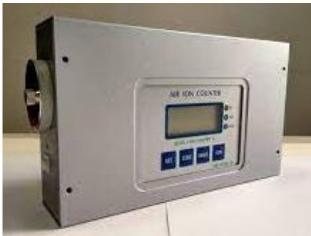
Figure 9: COM 3200Pro II ion meter used for ion measurements of the 30m 3 chamber.
